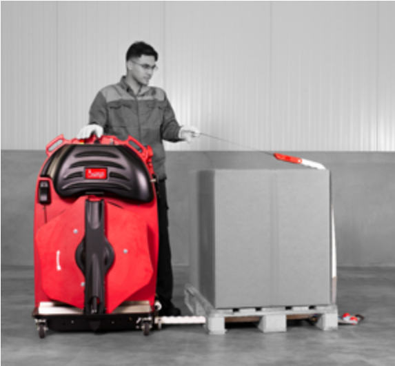
Up again on the rear side and over the pallet into the hand of the operator. The ChainLance retracts.
